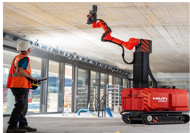
Figure 7: A Cobot Hilti machine collaborating with an employee (Hilti, 2020).
